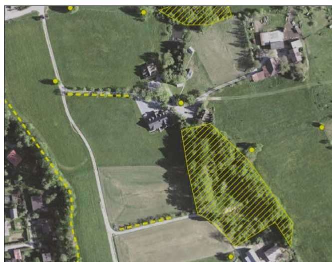
Fig. 10. Example of geometric representations of trees: area, line, point – class OT_PTLZ_A, class OT_OIPR_L and class OT_OIPR_P. WODGiK, 2017.
